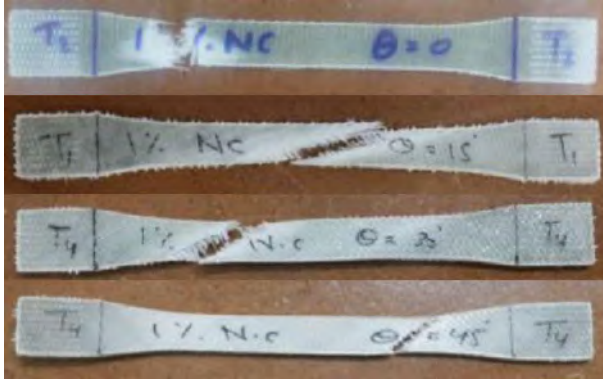
Figure 6. Specimens after tensile tests.
