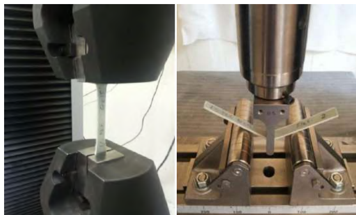
Figure 2. Mechanical Tests; a) Tensile test, b) Three point bending test.
