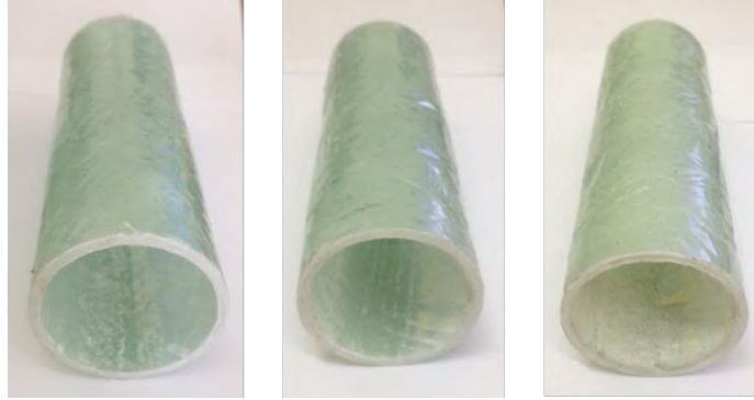
Figure 3. Specimens at different winding angle before test; a) 40°, b) 55°, c) 70°.
