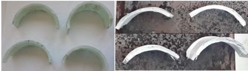
Figure 5. Examples of ignition loss specimens; a) before test, b) after test.
